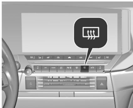
Wird durch Drücken von
