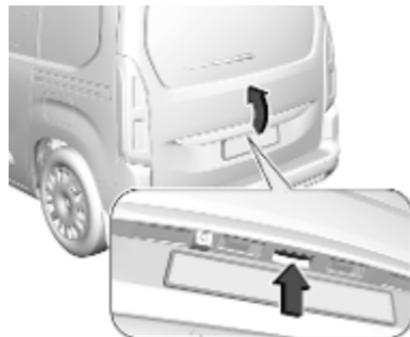
After unlocking, press the tailgate button and open the tailgate.
