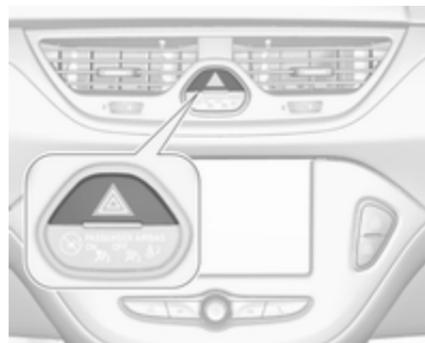
Wird durch Drücken von
