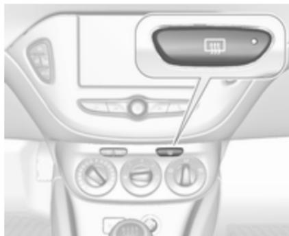
Wird durch Drücken von
