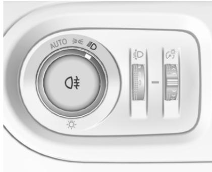
Wird durch Drücken von
