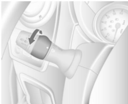
Inneren Schalter in Stellung
