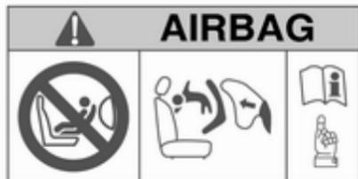
**EN:** NEVER use a rear-facing child restraint system on a seat protected by an ACTIVE AIRBAG in front of it, DEATH or SERIOUS INJURY to the CHILD can occur.
