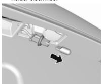
4. Pull the bulb out of the bulb holder and replace it.
