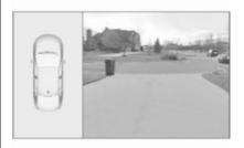
A view of the area in front of the vehicle may be displayed in the Info display. The front view is shown after shifting from **R** to **D** and when the vehicle is moving forward slower than 8 km/h.
