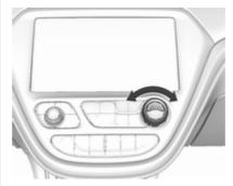
Set temperature to the desired value. The selected temperature is indicated in the display.
