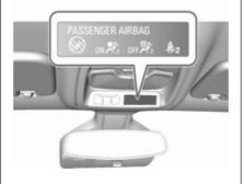
If control indicator ON illuminates for a certain time after the vehicle is switched on, the front passenger airbag system will inflate in the event of a collision.
