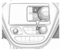
Press lower button to decrease or upper button to increase fan speed. The fan speed is indicated in the lower display area.
