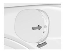
Push the rearward edge of the charge port door in and release to open the door.
