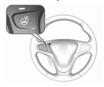
Activate heating by pressing 4. Activation is indicated by the LED in the button.
