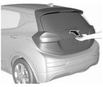
After unlocking, push the touchpad switch and open the tailgate.
