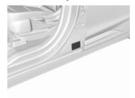
The identification plate is located on the front left or right door frame.
