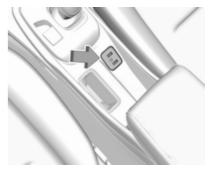
Two USB ports are located in the centre console. These ports can be used for charging and infotainment connection.
