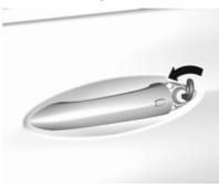
Manually unlock the driver's door by inserting and turning the key in the lock cylinder.
