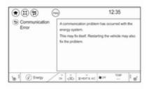
If a communication problem has occurred with the energy system, the error message is displayed. In this case, please try restarting the vehicle or contact a workshop.
