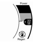
The power indicator gauge displays the instantaneous charge and discharge power flowing either into or out of the high voltage battery. Maximum discharge power is available when the high voltage battery is fully charged. During normal operation, a slight reduction in discharge power may occur as the high voltage battery state of charge decreases.
