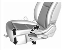
Lever pumping motion up : seat higher down : seat lower
