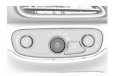
When the automatic light control function is switched on and the vehicle is switched on, the system switches between daytime running lights and headlights automatically depending on the external lighting conditions.
