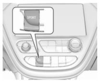
Sport mode provides more responsive acceleration than normal mode, but can reduce energy efficiency. Use normal mode whenever possible.
