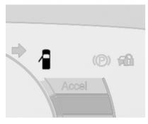
The indicator shows if a door, the bonnet or the tailgate is open. The symbol changes accordingly.
