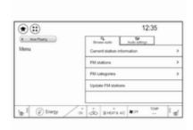
Select the **Browse audio** tab and then select the respective station list, e.g. **FM stations**. All receivable stations of the relevant waveband and in the current reception area are displayed.
