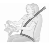
The seat belts are locked during heavy acceleration or deceleration of the vehicle, holding the occupants in the seat position. Thereby the risk of injury is considerably reduced.
