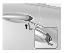
To remove the cap, press button at the back and extract the key blade from the housing. Insert the key into the recess at the bottom of the cap and swivel the key upward.
