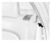
Guide the seat belts of the outer seats into the belt guides.
