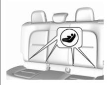
Fasten vehicle-approved ISOFIX child restraint systems to the ISOFIX mounting brackets. Specific vehicle ISOFIX child restraint system positions are marked in the ISOFIX table ♦ 53.
