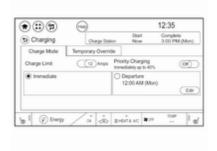
The vehicle starts charging as soon as it is connected to an electrical outlet.
