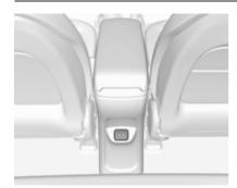
Another two USB ports for charging only are located in the back of the centre console.
