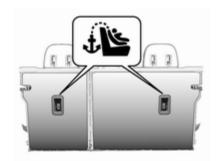
In addition to the ISOFIX mounting brackets, fasten the Top-tether strap to the Top-tether anchors.
