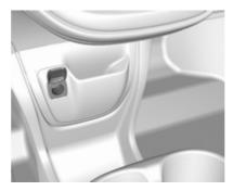
A 12 V power outlet is located in the centre console.
