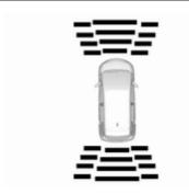
The distance indication can be inhibited by vehicle messages with a higher priority. After dismissing the message distance indication appears again.
