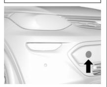
Wrap a cloth around the tip of a slot screwdriver to prevent paint damage. Insert the screwdriver in the slot at the
