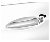
Push inside locking knob of all doors except driver's door or press in the driver's door panel. Then close the driver's door and lock it from the outside by turning the key in the lock cylinder. The charge port door and tailgate are possibly not locked.
