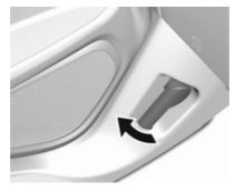
1. Pull the bonnet release lever and return it to its original position.
