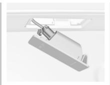
Remove the lamp housing from the bulb holder by turning the bulb holder clockwise.
