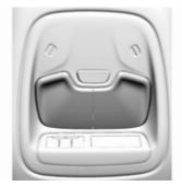
Operated by pressing the buttons at the front.
