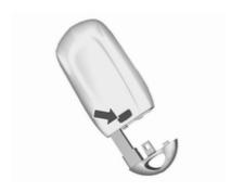
Press button at the back of the electronic key unit and extract the key blade from the housing.
