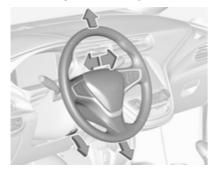
Unlock lever, adjust steering wheel, then engage lever and ensure it is fully locked.
