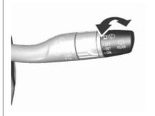
Turn outer cap to activate the rear window wiper:
