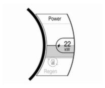
Regenerative power icon is shown as grey when regenerative power is limited. Additionally, a horizontal bar is displayed on the gauge. This usually occurs when the high voltage battery is near full charge or cold.
