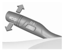
headlight flash : pull lever high beam : push lever low beam : push or pull lever
