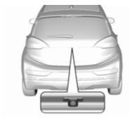
The camera is mounted between the number plate lights and has a viewing angle of 130°.
