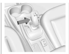
The release button is designed to prevent inadvertent shifting out of P unless the vehicle has been started. the brake pedal is depressed, and the release button is pressed.
