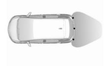
The system has three ultrasonic parking sensors in the rear bumper.
