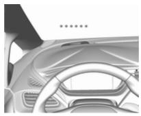
When the vehicle approaches a detected pedestrian ahead too rapidly, a red flashing LED alert is projected onto the windscreen in the driver's field of view and a warning chime is sounded. The brake system may prepare for driver braking to occur more rapidly which can cause a brief, mild deceleration. Continue to apply the brake pedal as required.
