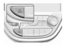
In the event of an accident with airbag deployment, the hazard warning flashers are activated automatically.
