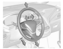
Unlock the lever, adjust the steering wheel, then engage the lever and ensure it is fully locked.
