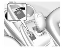
The electric parking brake can always be activated, even if the vehicle is switched off.
