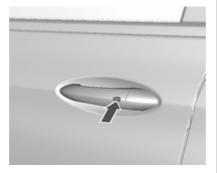
Press the button on any exterior door handle.
