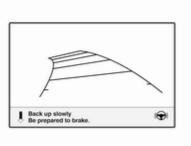
The parking slot suggestion of the system is accepted when the vehicle is stopped by the driver within 10 m for parallel parking slots or 6 m for perpendicular parking slots after the **Stop** message is given. The system calculates the optimal path into the parking slot.
