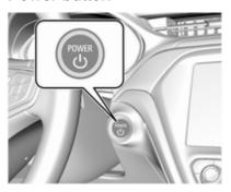
Electronic key must be inside the vehicle.
