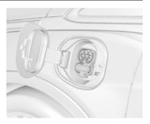
5. Plug in the vehicle plug of the charge cord into the charge port on the vehicle. Verify that the charging status indicator illuminates on top of the instrument panel and an audible beep occurs.
