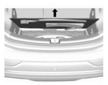
Lift up rear floor cover to gain access to the charge cord, vehicle tools and warning triangle.
