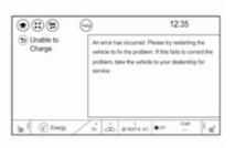
When the programmable charging system is disabled, the **Unable to charge** screen will be displayed.
