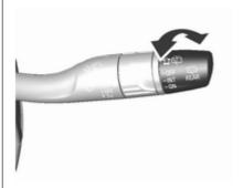
Turn outer cap to activate the rear window wiper:
