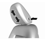
**Height adjustment**Press release button, adjust height, engage.
