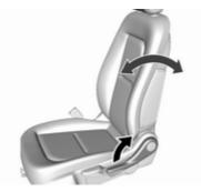
Pull lever, adjust inclination and release lever. Allow the backrest to engage audibly.
