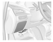
To open the compartment, compress the locking tabs, fold cover down and remove.
