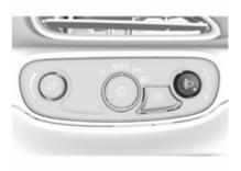
To adapt headlight range to the vehicle load to prevent dazzling: turn thumb wheel ∮ to required position.
