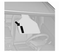
Keep the sensor free from dust, dirt and ice.
