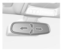
To adjust the mirror, move the mirror housing in the desired direction.
