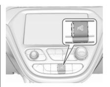
When searching for a parking slot, the system is ready to operate with a short press of ps.
