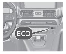
This mode adjusts the settings of the systems for a more economic fuel consumption, e.g. by optimising the automatic transmission shift points and adapting the sensitivity of the accelerator pedal.
