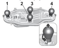
Push the bulb slightly down, turn it and remove it from the bulb carrier. Replace the bulb: Rear fog light (1) Reversing light (2) Turn light / hazard warning flasher (3) Tail light / brake light (4)
