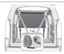
There are installation openings on both sides in the roof frame above the front seats. Open the covers and suspend and engage rod of net at one side, compress rod and suspend and engage at the other side.
