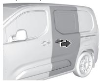
To open from inside push the handle and slide the door towards the rear beyond the point of resistance.
