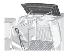
3. Move past the point of resistance to lock the ladder flap with the props.
