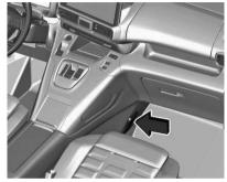
A 230 V power outlet may be located on the lower side of the centre console in the front passenger compartment. Do not exceed the maximum power consumption of 150 W.
