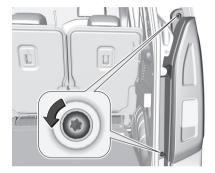
1. Unscrew and remove the two screws.
