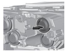
1. Remove the protective cover by pulling.
