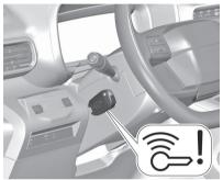
Hold the electronic key with buttons outside at the marking on the steering column cover as shown in the illustration. On vehicles with manual transmission, select neutral gear, operate the clutch pedal, the brake pedal and press **Start/Stop**.
