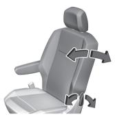
Push the lever, adjust inclination and release the lever. Do not lean on backrest when adjusting.
