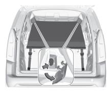
There are installation openings on both sides in the roof frame above the rear seats. Open the covers and suspend and engage rod of net at one side, compress rod and suspend and engage at the other side
