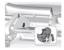
Turn the slider up or down in order to close or open the air vent.
