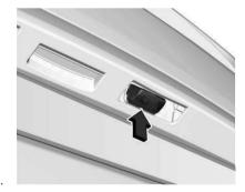
2. Insert a screwdriver in the recess of the cover and remove it.
