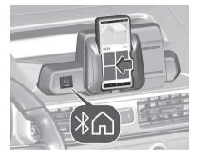
Pull the slide holder to the right, insert the mobile device into the support and fix it with the slide holder.
