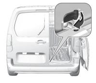
In exceptional cases only, it is possible to drive with the right-hand rear door open, e.g. if long objects need to be transported. Open the left-hand followed by the right-hand rear door, then close the left-hand rear door and lock it.
