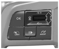
The set speed can be changed by moving the thumb wheel to to increase or to decrease thespeed. Move thumb wheel repeatedly to change speed in small steps, move and hold to change speed in large steps.
