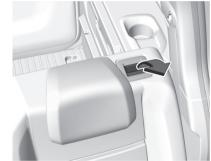
Pull the release lever on one or both outer sides and fold down the backrests onto the seat cushion.
