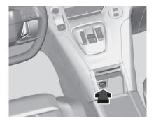
A 12 V power outlet is located behind the storage cover. Push cover upwards to open.
