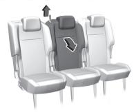
4. Depending on version, fold down the centre backrest by pulling the loop.
