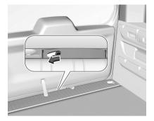
An access hole between the door and the floor enables the tailgate latch to be released using a suitable tool.
