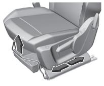
Pull the handle, slide the seat, then release the handle. Try to move the seat back and forth to ensure that the seat is locked in place.
