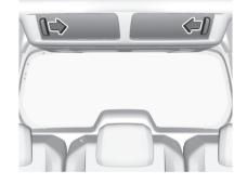
Slide the flaps to open. Close whilst driving. The maximum permitted load is **10 kg**.
