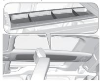
The separation of the four compartments can be taken out.
