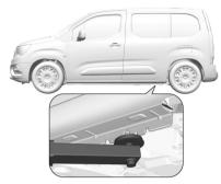
The rear arm position of the lifting platform is centrically under the relevant vehicle jacking point.
