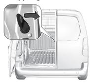
The right hand rear door is released using the lever.
