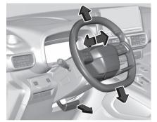
Unlock lever, adjust steering wheel, then engage lever and ensure it is fully locked. Do not adjust steering wheel unless vehicle is stationary and steering wheel lock has been released.
