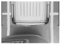
The camera records the vehicle's surroundings during the manoeuvre in order to reconstruct a view from above the vehicle in its near surroundings. Thus, the vehicle can be manoeuvred around obstacles nearby.
