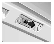
3. Pull the bulb from the bulb holder and replace it.
