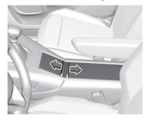
A storage box may be located in the centre console. Press cover to open. A 12 V power outlet is located behind the storage cover.
