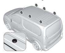
To fasten a roof rack, unscrew the caps in the roof strips. Insert the mounting provisions, as instructed, in the retainer.
