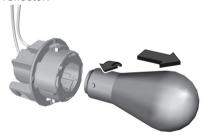
Rotate the lower bulb socket anticlockwise to disengage and detach the bulb.
