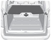
Pull the load compartment cover towards the rear and engage it in the side brackets.
