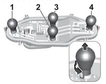
Push the bulb slightly down, turn it and remove it from the bulb carrier. Replace the bulb: Rear fog light (1) Reversing light (2) Turn light / hazard warning flasher (3) Tail light / brake light (4)
