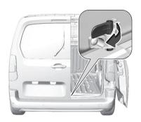
In exceptional case of transporting long objects in the load compartment with the need to have the right-hand rear door open, assure that the left door is closed and mechanically locked.
