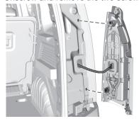
2. Carefully withdraw the tail light assembly from recess and remove.
