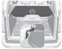
Remove load compartment cover from side brackets. Guide the cover until it is fully rolled up.
