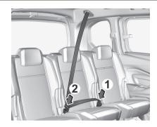
Insert lower latch plate into left-hand buckle (1) at the centre seat. Guide the upper latch plate with the seat belt over the lap area and the shoulder (do not twist) and insert it into right-hand buckle (2) at centre seat.
