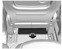
Vehicle tools may be located in the stowage compartments underneath the front seats
