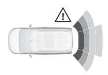
Additionally, the distance to rear obstacles is displayed by changing distance lines in the Info Display . When the obstacle is very close,  $\triangle$  for danger is displayed.
