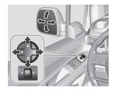
Select the relevant exterior mirror by pushing the mirror button  $\Box$  to the left or right.
