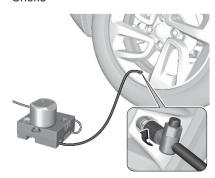
12 V compressor with cartridge of sealant and speed limit sticker. For temporary repair of a tyre and to adjust the tyre pressure.
