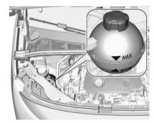
If the coolant level is at the **MIN** mark or below, seek the assistance of a workshop to have the engine coolant topped up.
