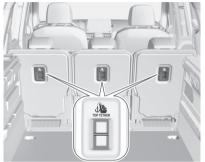
In addition to the ISOFIX brackets, fasten the top-tether strap to the top-tether anchors.
