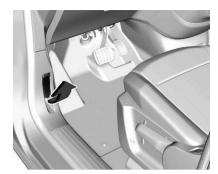
2. Pull the release lever and return it to its original position.
