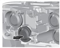
1. Remove the protective cover by pulling.
