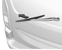
Lift the wiper arm. Disengage the wiper blade as shown in the illustration and remove.
