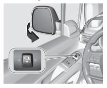
Pull the mirror button  $\square$  rearwards. Both exterior mirrors will fold. Pull the mirror button rearwards again to return both exterior mirrors to their original position.
