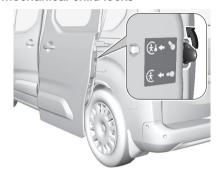
Turn the child lock in the rear door to the vertical position. The door cannot be opened from the inside.
