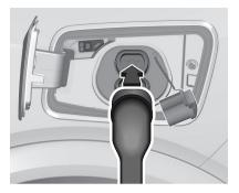
Plug in the vehicle plug of the charging cable into the charging port of the vehicle.
