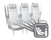
Fasten vehicle-approved ISOFIX child restraint systems to the ISOFIX brackets. Specific vehicle ISOFIX child restraint system positions are marked in the ISOFIX table.
