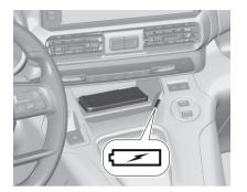
The portable device to be charged must be compatible with the Qi standard, either by design or by using a compatible holder or shell. The charging zone is identified by the Qi symbol.
