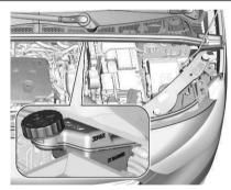
The brake fluid level must be between the **DANGER** and **MAX** marks. If fluid level is below **DANGER**, seek the assistance of a workshop.
