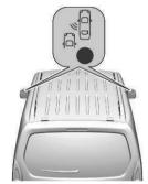
When the system detects a vehicle in the side blind zone while driving forwards, an LED will illuminate in the relevant exterior mirror.
