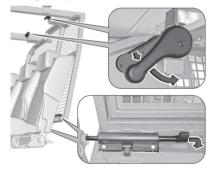
Release the four locking devices on the top and the bottom of the partition. 2. To be placed behind the front seats fold down the rear seat backrests
