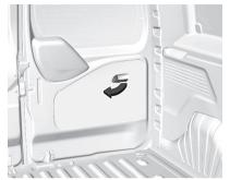
The door is opened from inside the vehicle by pulling the interior handle.
