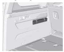
Depending on version, the warning triangle can be stowed in the load compartment. Secure it with the elastic straps.
