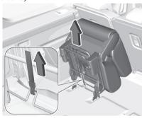
3. Pull the loop to disengage the locks and remove the seat assembly from the floor anchor points.
