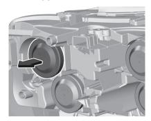
1. Remove the protective cover by pulling.
