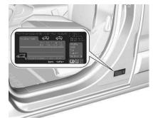
The tire pressure information label on the left door frame indicates the original equipment tires and the correspondent tire pressures.
