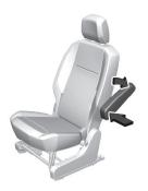
To remove the armrest fold it up, push and turn it to the position shown in the picture.
