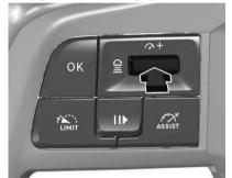
Press the button to display the current following distance setting in the Driver Information Centre.
