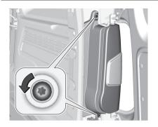
1. Unscrew and remove the two screws.
