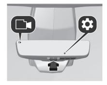
Press button to switch on and off. If activated, a camera symbol appears in the upper left corner.
