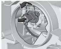
Disengage the spring clip from the retainer by moving it to the righthand side. Swivel the spring clip downwards. Withdraw the bulb socket from the reflector housing.
