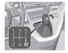
To engage reverse on 5-speed transmission, with the vehicle stationary
