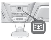
Press at the rear: the sunblind is opened as long as the switch is operated. Press at the front: the sunblind is closed as long as the switch is operated. No object should push the fabric against the roof.
