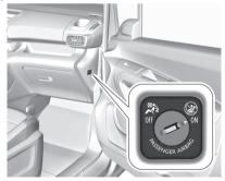
The front passenger airbag system can be deactivated via a key operated switch
