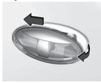
Slide the lamp housing forward and remove it at the back.
