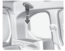
Pull latch plates with the seat belt out of seat belt holder in the roof.
