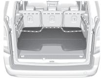
The rear parcel shelf can be installed in two positions.
