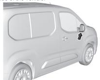
The camera is mounted at the bottom of the exterior mirror on the passenger side. The area displayed by the camera is limited. The distance of the image that appears on the display differs from the actual distance.
