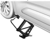
With the jack correctly aligned jack up until wheel is clear of the ground.
