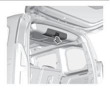
Pull handle to open. Close whilst driving. The maximum permitted load is **10 kg**.
