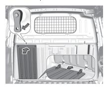
Turn the locking device upwards.
