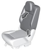
2. Pull the lever and fold down the backrest onto the seat cushion.
