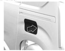
If the vehicle is equipped with an electronic key system, the fuel filler flap can only be opened if the vehicle is unlocked. Depending on the version,
