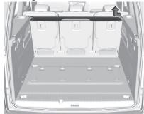
Open the load compartment cover. Compress the load compartment cover at one side and lift it up.
