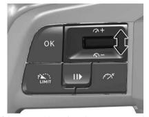
If the system is active, the preset speed can be changed by moving the thumb wheel to to increase or to decrease the speed. Move thumb wheel repeatedly to change speed in small steps, move and hold to change speed in large steps.
