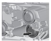
1. Remove the protective cover by pulling.
