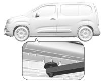
The front arm position of the lifting platform is centrically under the relevant vehicle jacking point.
