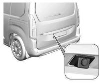
The camera is mounted in the rear bumper above the number plate.
