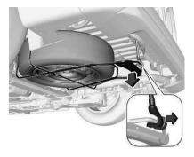
Lift the spare wheel holder and unhook the catch.
