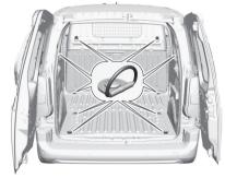
Lashing eyes may be located on the vehicle floor and / or in the sidewall.
