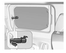
To partially open the rear windows, tilt the lever and push it fully to lock the windows in the open position.
