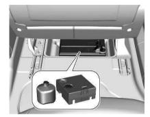
The tire repair kit is located in the storage compartment underneath the passenger front seat.
