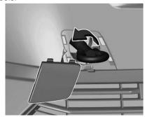
Screw in the towing eye as far as it will go, until it stops in a horizontal position. Attach a tow rope – or better still a tow rod – to the towing eye.
