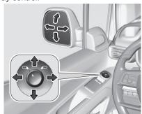
Select the relevant exterior mirror by turning the control to left  $\square$  or right  $\square$  mirror symbol .
