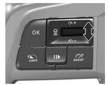
The preset speed can be changed by moving the thumb wheel to to increase or to decrease the speed. Move thumb wheel repeatedly to change speed in small steps, move and hold to change speed in large steps.
