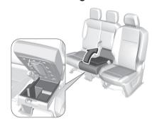
There may be a storage box under the centre bench seat. Lift up the seat cushion by pulling the handle. The storage box can be locked by a padlock.
