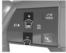
Press the button to display the current following distance setting in the cluster. Press the button successively to select the required following distance setting. The selected following distance is indicated by full bars on the adaptive cruise control screen.
