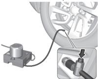
Drain excess tire pressure with the button on the air hose.
