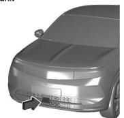
The radar unit is located in the middle of the front bumper.
