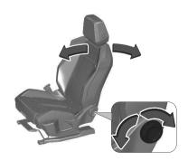
Rotate the wheel forwards or backwards to recline the seat.
