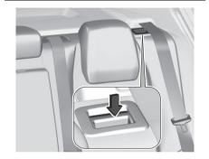
The backrests are properly engaged when the red marks near the release levers are no longer visible.
