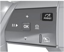
Press successively until the adaptive cruise control mode is selected. The adaptive cruise control screen is displayed. The system is still not activated.
