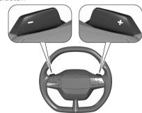
Pull left paddle - to increase the braking force and pull right paddle + to decrease. Use the maximum braking force when driving down steep hills, in deep snow, in mud or in stop-and-go traffic. The braking level setting is saved when ignition is switched off. Regenerative Braking ⇒ page 115
