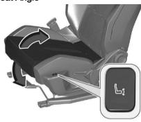
Press and hold the front or rear of the button to adjust the angle.
