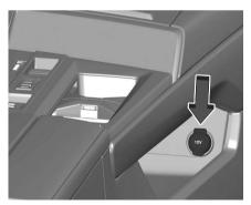
A 12 V power outlet is located in the front centre console.
