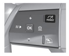
Press at the steering wheel successively until the Drive Assist mode is selected.
