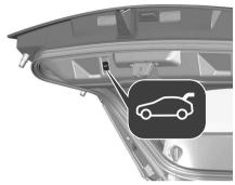
To close, press sin the open tailgate until the tailgate starts to move.
