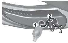
Close the lock using the key by turning it anti-clockwise and pulling it.
