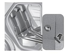
ISOFIX brackets are indicated by a label on the backrest. To get access to the ISOFIX brackets, first pull the zipper. An i-Size child restraint system is an universal ISOFIX child restraint system according to UN Regulation No. 129. All i-Size child restraint systems can be used on any vehicle seat suitable for i-Size, child restraint installation table ⇒ page 37.
