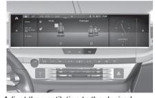
Adjust the ventilation to the desired intensity by pressing for the respective seat one or more times. The control indicator in the button indicates the selected intensity.
