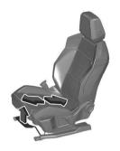
Pull handle, slide seat, release handle. Try to move the seat back and forth to ensure that the seat is locked in place.
