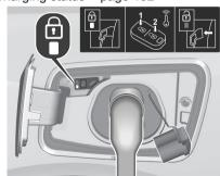
Once charging, the vehicle plug will be locked to the charging port and cannot be
