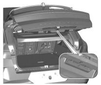
Stow the warning triangle in the space at the rear of the trunk door and secure it with the Velcro® fastener.
