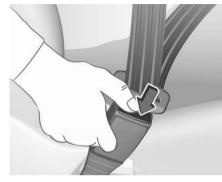
To release seat belt, press red button on seat belt buckle and guide the seat belt back.
