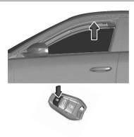
Press and hold to close the windows. Release the button to stop window movement.
