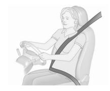
The seat belts are locked during heavy acceleration or deceleration of the vehicle, holding the occupants in the seat
