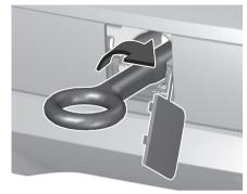
Screw in the towing eye as far as it will go until it stops in a horizontal position. Attach a tow rope – or better still a tow rod – to the towing eye.
