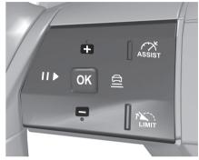
The preset speed can be changed by pressing + to increase or - to decrease the speed. A short press changes speed by 1 km/h, a long press changes speed by 5 km/h.
