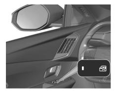
Press the button to deactivate the rear door power windows; the LED illuminates. To activate, press again.
