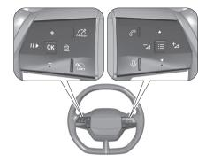
Some driver assistance systems, the Infotainment system and a connected mobile phone can be operated via the controls on the steering wheel.
