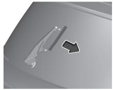
Lift wiper arm. Disengage wiper blade as shown in illustration and remove. Attach the wiper blade slightly angled to the wiper arm and push until it engages. Lower wiper arm carefully.
