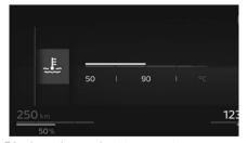
Displays the coolant temperature.
