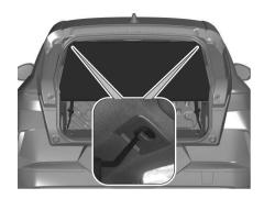
There are installation openings on both sides in the roof frame above the rear seats: suspend and engage rod of net at one side, compress rod and suspend and engage at the other side.
