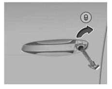
Manually lock the left front door by inserting and turning the key in the lock cylinder. With working central locking system the vehicle will be locked
