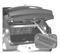
Stow the warning triangle in the space in the tailgate and secure it with the Velcro® fastener.
