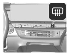
Press the button to activate the function. The heating switches off automatically after a certain time depending on the outside temperature.
