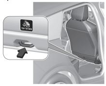
Top-tether anchors are marked with a symbol for child seat.
