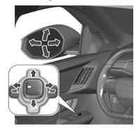
Select the relevant exterior mirror by turning the control.
