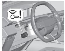
Hold the electronic key at the marking on the steering column cover as shown in the illustration. On vehicles with manual transmission, select neutral gear, operate the clutch pedal, the brake pedal and press **Start/Stop**.
