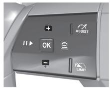
The set speed can be changed by using the buttons to + to increase or - to decrease the speed. Move thumb wheel repeatedly to change speed in small steps, move and hold to change speed in large steps.
