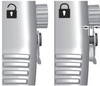
Make sure the mechanism is unlocked (only red mark is visible).
