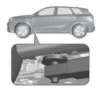
The front arm position of the lifting platform is centrically under the relevant vehicle jacking point.
