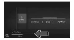
Displays the high voltage battery state of charge.
