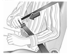
Withdraw the seat belt from the retractor, guide it untwisted across the body and insert the latch plate into the buckle. Make sure the seat belt lies across the shoulder and fits tightly to the body while driving.
