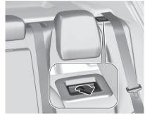
Pull the release lever and fold down the backrests onto the seat cushion.
