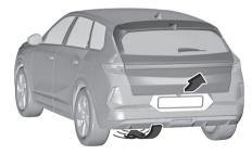
To open or close the tailgate, move the foot back and forth in the area shown in the illustration. Do not hold the foot longer or move too slow below the bumper. The electronic key must be outside the vehicle, within a range of approx. 1 m of the tailgate. The turn lights will flash to indicate the
