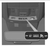
If the control indicator ON illuminates for approx. 60 seconds after the ignition is switched on, the front passenger airbag system will inflate in the event of a collision.
