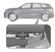
The rear arm position of the lifting platform is centrically under the relevant vehicle jacking point. On BEV vehicles, there is a protective cover that must be removed first.
