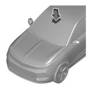
Do not attach stickers such as toll road stickers or similar on the windscreen in the area of the interior mirror. Keep the sensor free from dust, dirt and ice. Otherwise, the detection zone of the rain sensor / light sensor and the view area of the camera in the mirror housing could be restricted. ⇒ page 44
