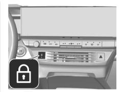
Press to lock. The LED in the button illuminates.
