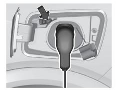
The start of charging is indicated by the green flashing of the status indicator at the charging port and at the control box of the charging cable if available.
