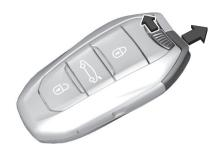
To eject the key or put it back in place, pull and hold the button.
