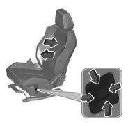
Adjust lumbar support using the four-way switch to suit personal requirements. Press and hold the front or rear of the switch to increase or decrease the lumbar support.
