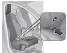
Fasten vehicle-approved ISOFIX child restraint systems to the ISOFIX brackets. Specific vehicle ISOFIX child restraint system positions are marked in the child restraints table.
