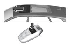
Press and hold for more than two seconds to close the sunroof. Release the button to stop the movement.
