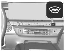
Press the button to activate the function. The heating works only with freezing outside temperatures and switches off automatically after a certain time depending on the outside temperature.
