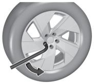
Attach the wheel wrench and loosen each wheel bolt by half a turn.
