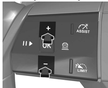
Press the button to display the current following distance setting in the cluster.
