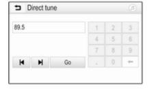
Enter the desired frequency. Use ← to delete digits entered. If necessary, touch
