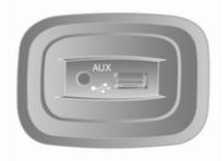
Depending on version, in the Infotainment unit (or on the instrument panel) there is an AUX socket for the connection of external audio sources.
