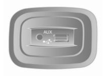
Depending on version, in the Infotainment unit (or on the instrument panel) there is a USB socket  $\psi$  for the connection of external audio sources.
