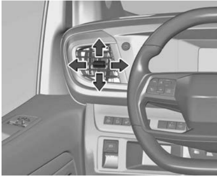
Outer air vents in the instrument panel
