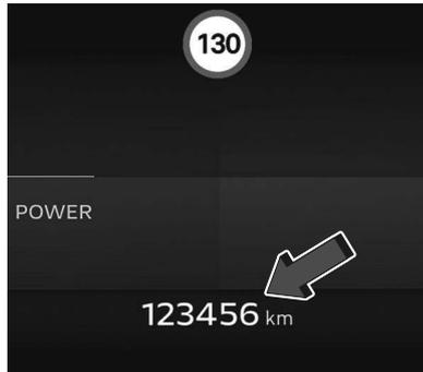
The total recorded distance of the vehicle is displayed in the right bottom corner of the cluster (MHEV/PHEV), or the bottom left corner (BEV).
