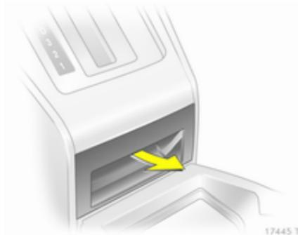
2. Extraire l'élément de cendrier
