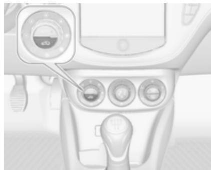
Za vklop kroženja zraka pritisnite
