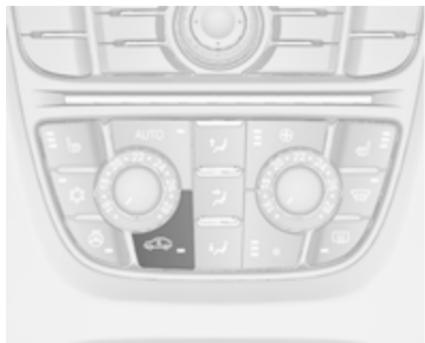
Za vklop kroženja zraka pritisnite gumb
