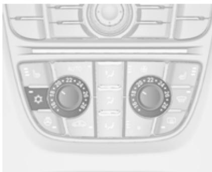
Za vklop hlajenja pritisnite tipko
