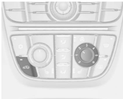
Za vklop kroženja zraka pritisnite gumb
