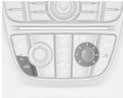
Za vklop kroženja zraka pritisnite
