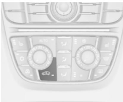
Za vklop kroženja zraka pritisnite
