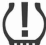
Če sistem zazna nizek tlak v pnevmatikah, sveti kontrolna lučka
