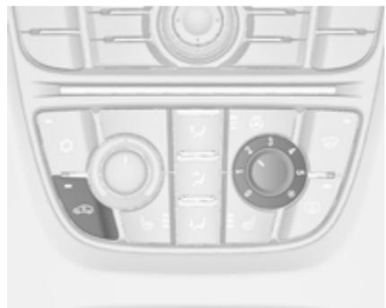
Za vklop kroženja zraka pritisnite gumb
