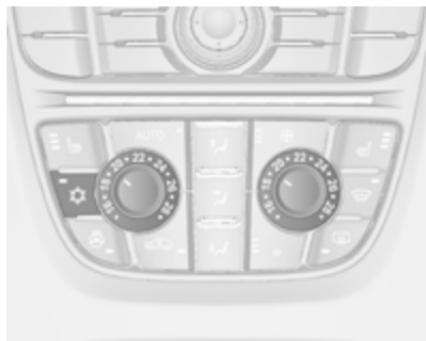
Za vklop hlajenja pritisnite tipko
