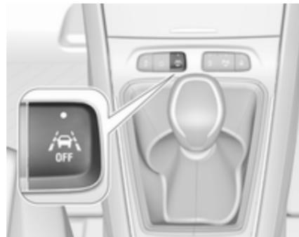
Če je sistem vklopljen, lučka LED v gumbu
