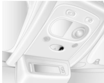
Za odklepanje ali zaklepanje vrat pritisnite gumb
