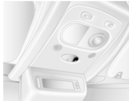
Za zaklepanje ali odklepanje pritisnite stikalo
