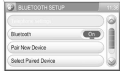
Za odpiranje menija **BLUETOOTH SETUP (BLUETOOTH NASTAVITEV)**: pritisnite gumb **SETUP**, nato pa izberite element menija **Bluetooth & telephone (Bluetooth in telefon)**.
