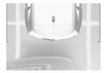
The camera records the vehicle's surroundings during the manoeuvre in order to reconstruct a view from above the rear of the vehicle in its near surroundings, allowing the vehicle to be manoeuvred around
