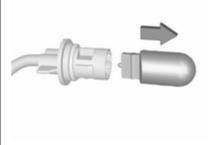
3. Pull bulb from bulb holder and replace it.
