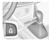
Remotely operated system to prevent opening of the rear doors using their interior controls and use of the rear electric windows.
