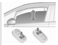
Press and hold to open windows. Press and hold to close windows. Release button to stop window
