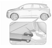
Rear arm position of the lifting platform at the underbody.
