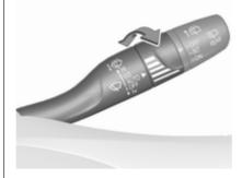
Wiper lever in position **AUTO**. Turn the adjuster wheel to adjust the sensitivity of the rain sensor.
