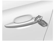
Manually lock the driver's door by inserting and turning the key in the lock cylinder.
