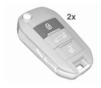
Press <sup>®</sup> on the radio remote control twice within five seconds.
