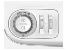
When the automatic light control function is switched on and the engine is running, the system switches between daytime running lights and headlights automatically depending on the external lighting conditions and information given by the rain sensor system.
