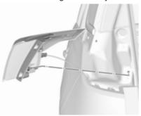
2. Remove the light assembly by pulling it straight back.
