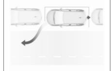
Move forwards and backwards while observing the warnings of the Parking assist until the end of manoeuvre is indicated. The manoeuvre is complete when the vehicle's front wheels are out of the parking slot and  $P_{\Theta}$  extinguishes in the instrument cluster.
