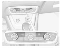
Set the preselected temperatures separately for driver and front passenger to the desired value using the left and right control dials. The dial on the passenger side changes the temperature for the passenger side. The dial on the driver's side changes the temperature for the driver's side or for both sides depending on activation of synchronisation MONO in the climate settings menu. Press MENU to enter the menu.
