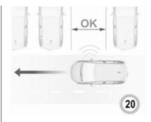
When a free slot is detected, a visual feedback on the Colour-Info-Display and an acoustic signal is given. Stop the vehicle, select reverse gear, release the steering wheel and start moving without exceeding 4 mph.
