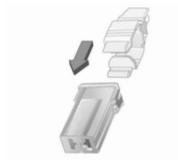
Place the fuse extractor on the various types of fuse from the top or side, and withdraw fuse.
