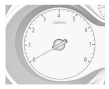
Displays the engine speed.
