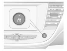
You can activate or deactivate this function permanently. With the ignition on, press \( \text{\text{\text{d}}} \) until an audible signal starts and a corresponding message is displayed.
