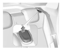
To fold down the backrest from the load compartment, lift the release lever.
