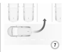
Move forwards and backwards as instructed by observing the warnings of the Parking assist and paying attention to the acoustic signals until the end of manoeuvre is indicated. When finished, Pa extinguishes in the instrument cluster.
