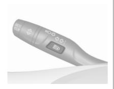
Activate this function pressing a button on the turn and lane change lever. The LED of the button illuminates if the high beam assist is activated. The high beam is switched on automatically at a speed above 15 mph.
