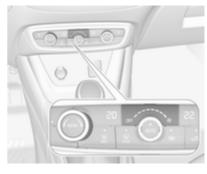
Adjust the air flow by turning rotary knob % to the desired speed. Turn left to decrease or turn right to increase. Fan speed can also be changed by touch buttons in the climate settings display. Press **MENU** to enter the menu.
