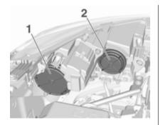
High beam, turn signal light (1) Low beam (2)
