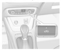
Press to activate air recirculation mode, LED is indicated.
