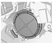
1. Rotate the cap (1) anticlockwise and remove it.
