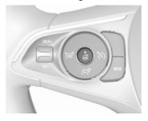
Activate heating by pressing **3**. Activation is indicated by the LED in the button.
