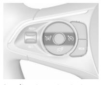
Press © on the steering wheel: symbol © and Pause are indicated in the Driver Information Centre. The system is still not active.
