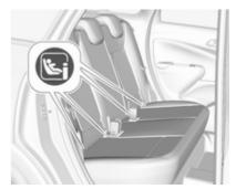
Fasten vehicle-approved ISOFIX child restraint systems to the ISOFIX brackets. Specific vehicle ISOFIX child restraint system positions are marked in the ISOFIX table ⋄ 60.
