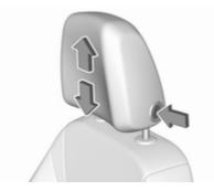
Press release button, adjust height, engage.
