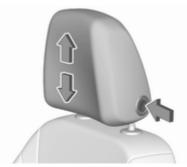
Press release button, adjust height, engage.
