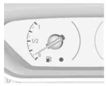
Displays the fuel level in the tank.
