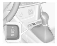
The lane departure warning system is activated by pressing \( \mathbb{\mathbb{L}} \). The system is switched on when the LED in the button is not illuminated.
