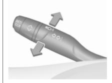
headlight flash : pull lever high beam : push lever low beam : push or pull lever
