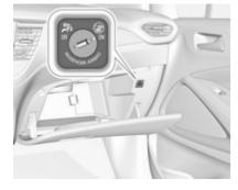
The front passenger airbag system can be deactivated via a keyoperated switch on the passenger side of the instrument panel. Use the ignition key to choose the position:
