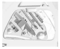
The jack, tools, a strap for securing a damaged wheel and the towing eye are placed in the tool box in the right wall of the load compartment. Spare wheel ♀ 214.
