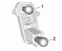
Remove the bulb by pulling and replace.
