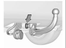
Attach breakaway stopping cable to eve.
