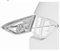
Carefully withdraw the light assembly from the recesses and remove.
