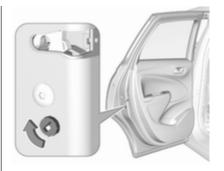
To lock the other doors, first remove the black cover by inserting a key and turning clockwise.
