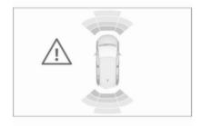
Additionally, the distance to rear and front obstacles is displayed by changing distance lines in the Info-Display ♀ 97.
