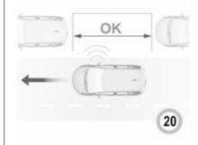
When a free slot is detected, a visual feedback on the Colour-Info-Display and a first acoustic signal is given. Drive slowly forwards. When the second acoustic signal is given, stop the vehicle, select reverse gear, release the steering wheel and start moving without exceeding 4 mph.
