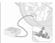
16. Continue driving immediately so that sealant is evenly distributed in the tyre. After driving approx. three miles (but no more than ten minutes), stop and check tyre pressure. Screw compressor air hose directly onto tyre valve when doing this. Fill tyre as described before. Drain excess tyre pressure with the button on the air hose.
