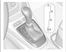
Move the selector lever in the shifting gate as shown in the illustration above.
