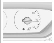
Displays the coolant temperature.
