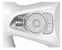
Accelerate to the desired speed and press toggle switch once briefly to RES/+ or SET/-. The current speed is stored and maintained. Accelerator pedal can be released.
