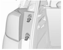
Unscrew the two screws that secure the light assembly.
