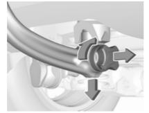
Open the protective flap and turn the key to position do unlock the coupling ball bar.
