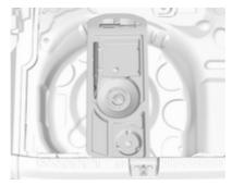
The screwdriver and the towing eye are located in a box below the floor cover in the load compartment.
