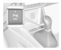
The system is switched off when reverse gear is disengaged. Press P<sup>\*</sup> OFF to deactivate the system manually. The LED in the button illuminates when the system is deactivated.
