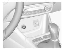
The cigarette lighter is located is located behind the storage cover below the climate controls. Press cover to open.
