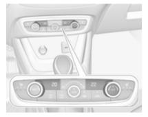
Press **A/C** to switch on cooling. The LED in the button illuminates to indicate activation. Cooling is only functional when the engine is running and climate control fan is switched on. Press **A/C** again to switch off cooling.
